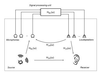
Fig. 3: Schematic drawing of an active acoustic system (cf. [6]).
