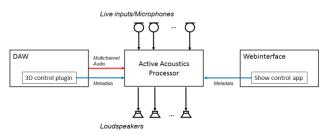
Fig. 5: 3D Audio production chain for recorded and live inputs.
