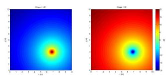
**Fig. 4:** Distribution of relative sound level from a microphone to loudspeakers across a 10x10m room. Top: Natural decay of level over distance (Shape =  $\pm 20$ ). Bottom: Less decay of level over distance (Shape =  $\pm 10$ ).
