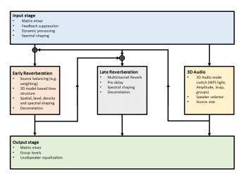
Fig. 6: Signal processing framework for an Active Acoustic system.
